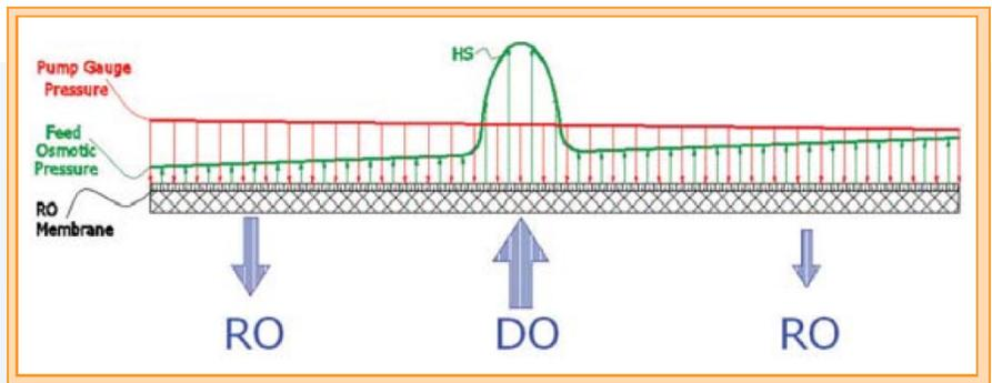
In the clean-in- place tank, a 25% saline solution is added with an osmotic pressure of 2800 psi. For 10 - 15 seconds, this saline solution is injected into the feed water stream. The osmotic pressure is much higher than the hydrostatic pressure of the feed water pump, reversing the osmotic flow and back washing each membrane in succession like a vacuum cleaner.
